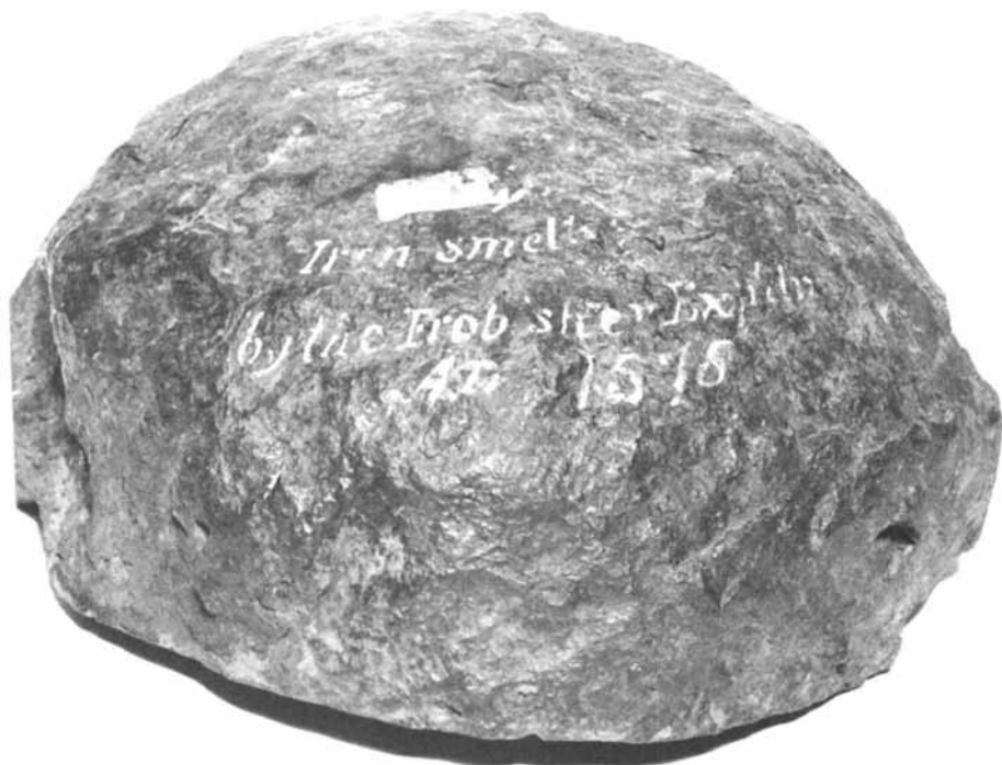
Figure 1. An iron bloom in the collection of the Department of Naval History, National Museum of American History, Smithsonian Institution (Cat. No. 49459). The bloom weighs approximately 17 lb, after sampling, and is approximately 18 cm in diameter on the base as shown. (Smithsonian Institution negative No. 74836.)
